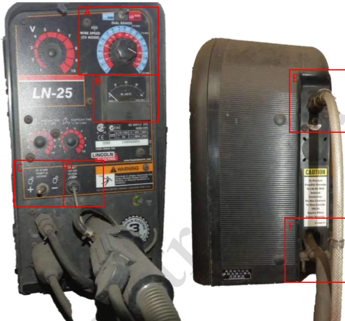
Gambar 3. Penjelasan panel Wire Feeder Lincoln LN25
